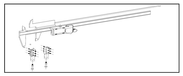
2. Pair of anvil with disc Available disc diameter Ø 6 / Ø10 / Ø12.5
