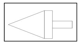
4. Pair of anvil with cylindrical surface 1.5 mm
